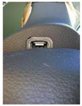
Use a mirror to see a hole on the back of the stering wheel. In that hole you can see one of the airbag retaining loops.
