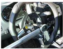
Undo the steering wheel mounting bolt. If you don't have the special 12-star bit, a regular six-star Torx bit (T55) will do just fine.
