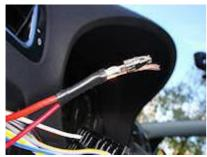
Connect the new wire coming from te slip ring / stalk switch unit pin 9.
