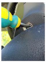
Use a flathead screwdriver to lever the retaining loop around the stud on the steering wheel. Simultaneously, pull from the edge of the airbag towards you.
