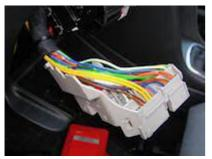
Push the ends of the repair wires into their designated positions. Make sure the locking tabs on the pins engage with connector body so the wires don't become loose later.
