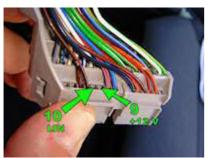
Under the cover you can see the individual wire positions in the connector body. You'll need to add the ends of the repair wires to positions 9 and 10 indicated by the arrows.
