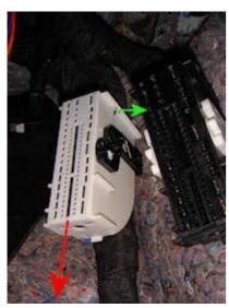
The connector cover is removed by spreading the locking tabs on both sides in the direction of the green arrow, while simultaneously pulling the cover in the direction of the red arrow.
