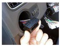
Light switch removed and its connector exposed.
