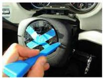
Push the steering column upper trim half from both sides as shown to unclip it from the lower trim half.
