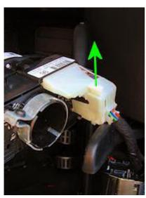
Undo the connector T41 at the slip ring / stalk switch. There's a locking to the connector: lift up the locking rod as indicated by the green arrow.
