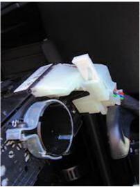
Locking rod completely up, the connector is free to come off.
