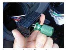
Free the pin 15 from the connector body using an approriate tool, or alternatively by pushing with
