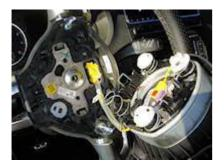
Hold the airbag in your other hand to prevent it hanging from the wiring. Undo the yellow connector that goes to the slip ring. Pull the white locking piece towards you to free the connector.
