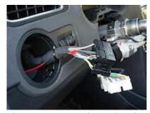
The new wire in place. Shrink tubing and a wire tie used to secure the new wire.
