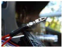
The new wire soldered to the base of the pin. Try to make the join as thin as possible, otherwise you may have trouble getting the pin to fit back into the connector body. Be careful not to destroy the dashboard with the hot soldering iron!
