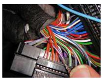
Free the violet-white wire from the connector body position 17. It should free using roughly the same method as for the light switch connector before. Then you can remove the insulation from around the copper wire for connecting the new wire.
