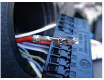
The pin freed. You can see the small locking tabs you need to push down for the pin to come out.
