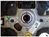
Turn the wheels and steering wheel back to straight-ahead position. Always a good practice to mark the position of the steering wheel in relation to the end of the steering axle, even if you weren't to mount the same wheel back on this car.
