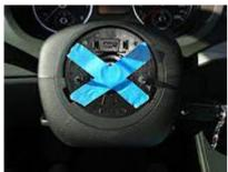
Now you can see the airbag slip ring that makes all the electrical connections to the steering wheel. Avoid spinning the slip ring, otherwise you might lose its central position, which could lead to the ribbon cable getting destroyed the next time you turn the steering to full lock. Use tape to "lock" the slip ring to this central position.
