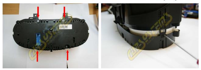
Unscrew four T8 bolts Remove front cover of instrument cluster. Attach new cover.
