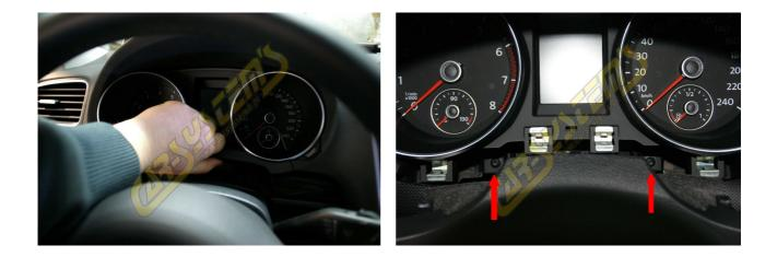
To remove instrument cluster in VW golf mk6, pull out small plastic piece under cluster. Unscrew two T25 bolts marked on pic2 and pull out whole cluster unit.
