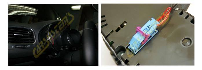
Make sure that ignition is OFF Remove blue plug from cluster Remove Instruments cluster from car
